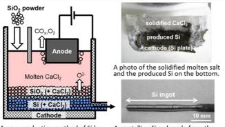
A new production method of Si by molten salt electrolysis.
