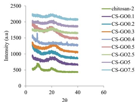
Fig 3 XRD patterns of chitosan and CS-GO composites
